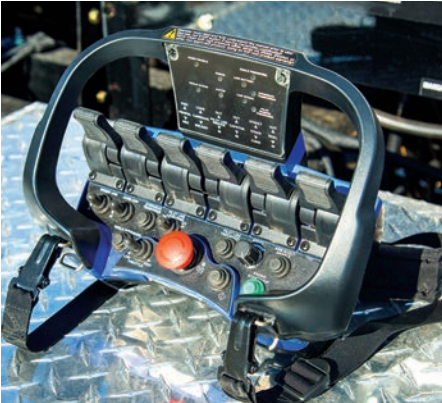
RADIO REMOTE WITH MAXIMIZED FUNCTION CONTROLS
