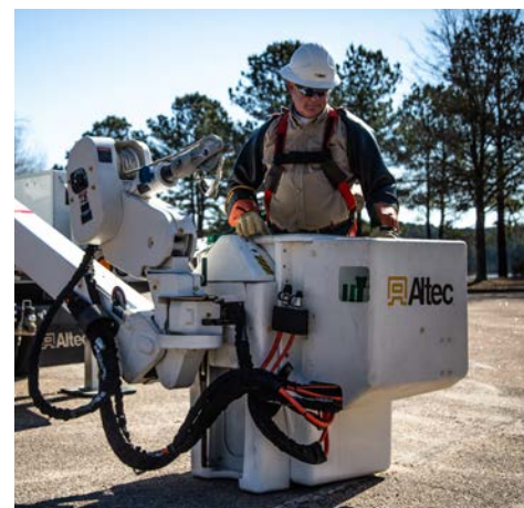
24 INCH PLATFORM ELEVATOR OPTIMIZES OPERATOR REACH WITHIN WORK ZONE
